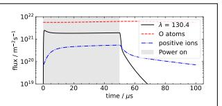
**Fig. 1.** Fluxes of O atoms, positive ions and VUV photons to surfaces during a single pulse cycle. Conditions: 100% O<sub>2</sub>, pressure = 5 Pa, pulse-averaged power = 400 W, pulse repetition frequency = 10 kHz, duty cycle = 50%
